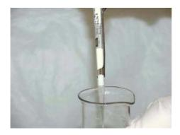
m) Touch pipette against wall of delivery vessel at correct angle (see 4.2). Be careful to not immerse tip in any liquid already in receiving vessel.
