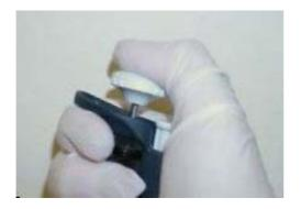
f) Expel the contents of the pipette by pressing the plunger down steadily and evenly to first stop position while keeping the tip in contact with the wall of the vessel. Wipe the tip for 8 mm to 10 mm to remove any remaining liquid.
