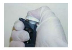
g) Push plunger down to second stop. This will force air through the tip to expel any remaining liquid.
