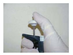
d) Ensure that the plunger extends fully to its upper stop position and wait one or two seconds before withdrawing the tip of the pipette from the liquid.
