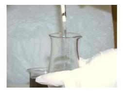
e) Touch the pipette against the wall of receiving vessel at an angle of about 30° to 45°. Be careful to not immerse the tip in any liquid already in the receiving vessel.
