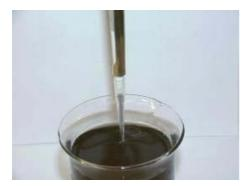
c) Immerse the tip of the pipette in liquid to the correct depth (see 4.2 and Table 1).Keep the pipette in a vertical position and release the plunger in a smooth and uniform manner to aspirate the liquid.
