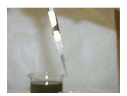
n) Note that some liquid will be left in the tip after dispensing. This should be returned to the original vessel.
