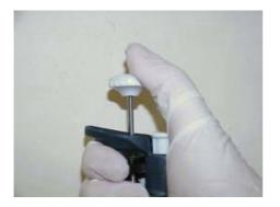
k) Ensure that the plunger extends fully to its upper stop position. Check the tip to make sure no drops are forming at the orifice.
