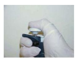
b) Press the plunger down smoothly to the first stop position. At this stage the pipette tip must not be immersed in the liquid.
