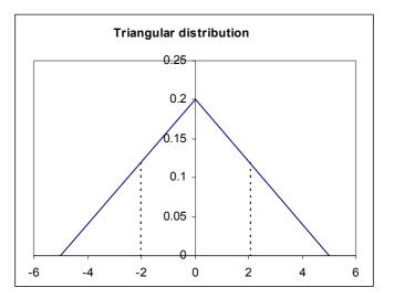
Figure 6. Triangular distribution, with a mean value of zero and limits  $\pm 5$ . One standard deviation is  $\pm 2.04$ .
