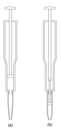
Figure 1. Schematic cross sections of (a) air displacement pipette and (b) positive displacement pipette
