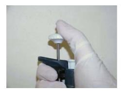
a) Attach tip to tip holder taking care to avoid contamination. Hold pipette comfortably in one hand with thumb resting on plunger.
