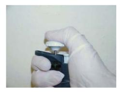
Touch tip against wall of receiving vessel and expel the contents of the pipette by pressing the plunger down steadily and evenly, but only to the first stop position.
